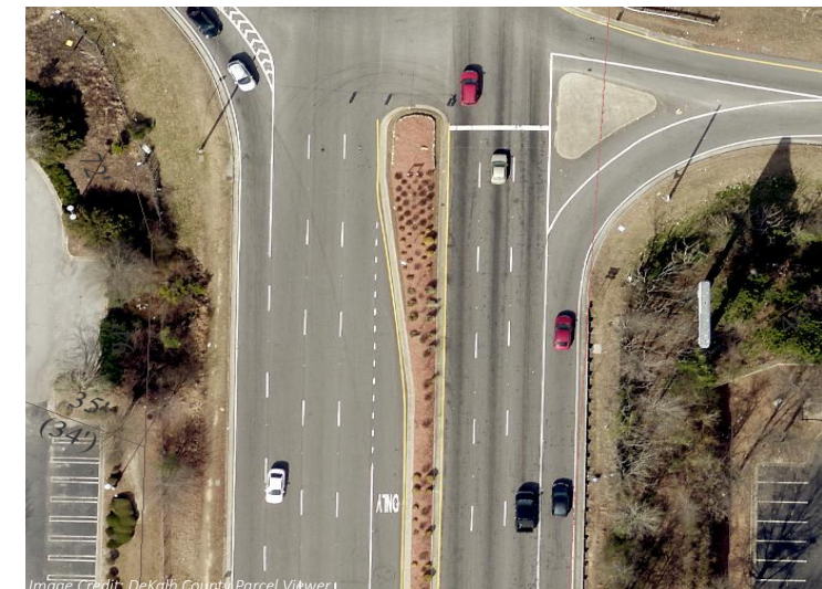
AERIAL VIEW SHOWS DESIRE LINES ON BOTH SIDES OF THE ROAD, ESPECIALLY THE WEST SIDE
