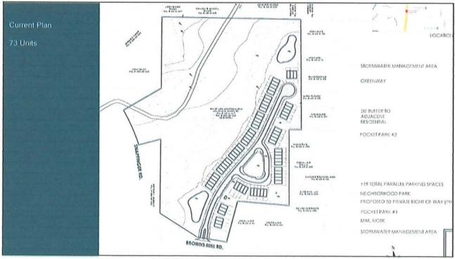
SUMMARY: CURRENT ZONING: RSM GROSS ACREAGE...... USEABLE AREA\*... DEVELOPED AREA... .....±5.5 AC ROADS (1.9 AC) + LOTS (3.6 AC) TOTAL OPEN SPACE PROVIDED...... ... 19.4 AC GROSS ACREAGE [124.9 AC] - DEVELOPED AREA [15.5 AC] 1, SETBACKS ARE 20' FRONT, 15' REAR, WITH 10' MINIMUM BUILDING SEPARATION. 1, SEIBACKS ARE 20' FRONT, 15' REAR, WITH 10' MINIMUM BUTCHING SEPARATION,
